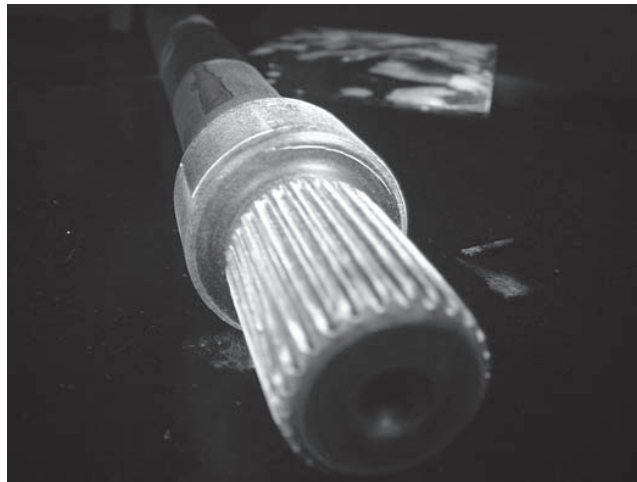
FIG. A1.1 Axle with Circumferential Crack in Shoulder
