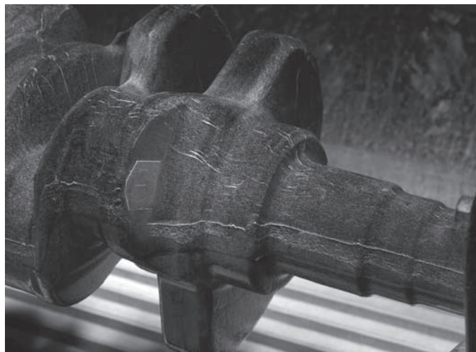
FIG. A1.4 Crankshaft with Various Longitudinal Indications
